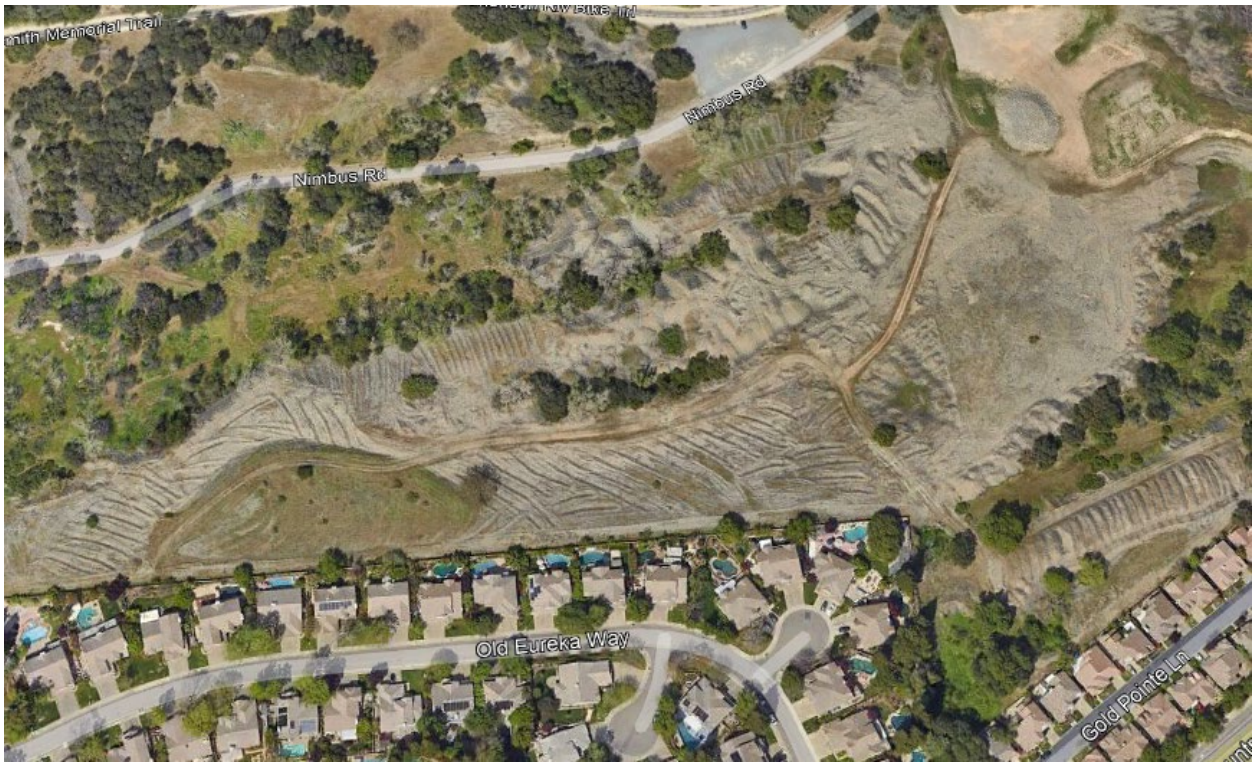
Figure 6: Hydraulic mining tailings serve as fuel breaks between Gold River and the Nimbus Fish Hatchery. (Map Imagery ©2023 Google, 2022 CNES / Airbus, Maxar Technologies, U.S. Geological Survey)
